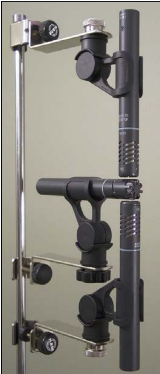
Photo 1: Daniel Courville assembled this first-order B-format microphone array, which uses an AKG SE300B-CK92 omni and a pair of AKG SE300B-CK94 figure eights. These microphones were chosen because they have the same sensitivities. For “above” and “below” pickups, another figure-eight microphone would need to be placed horizontally parallel to the omni.
