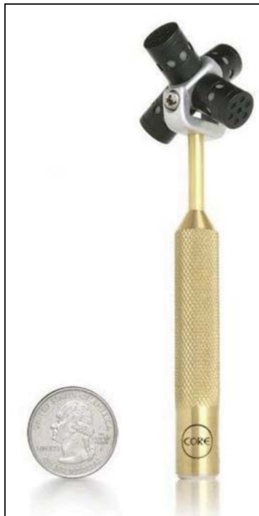
Photo 1: Daniel Courville assembled this first-order B-format microphone array, which uses an AKG SE300B-CK92 omni and a pair of AKG SE300B-CK94 figure eights. These microphones were chosen because they have the same sensitivities. For “above” and “below” pickups, another figure-eight microphone would need to be placed horizontally parallel to the omni.
